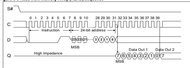
The instruction is not accepted, and is not executed, if a Write cycle is currently in progress.
