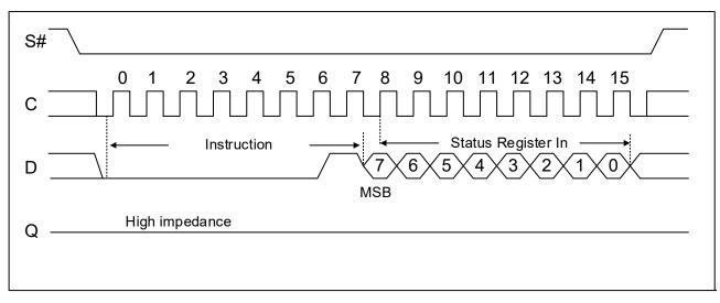
Driving the Chip Select (S#) signal high at a byte boundary of the input data triggers the self-timed Write cycle that takes tW to complete (as specified in AC tables in: DC and AC parameters).
